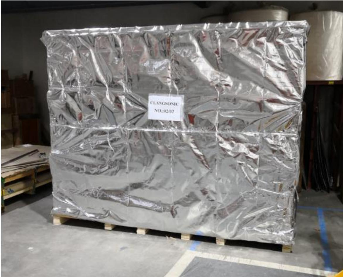
The packing is adopting exportable wooden box or pallet, wrapped with moisture-proof material which can protect the machine from dust and moisture during sea shipment.
